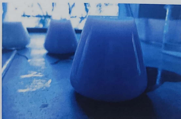
Fig 11: Colour change from light pink to purple it shows presence of calcium.
